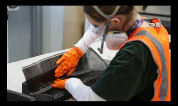
One of the key milestones this year has been securing the resources necessary to produce a complete carbon composite bodywork package. This advancement enables significant weight reduction and improved rigidity across the car's surfaces. Staying true to the aesthetic identity established in 2023 and 2024, this year's car will once again showcase raw 4x4 twill carbon with the distinctive V-seam pattern extending down the length of the vehicle—even into the footwells.
